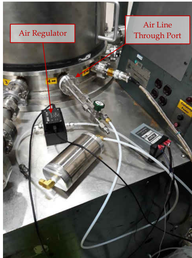
Fig. 29 Location of through port for the air line coming from the air regulator.
