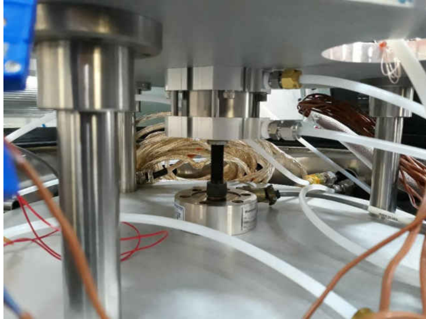
Fig. 32 Placement of air cylinder and load cell.
